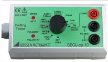
All limit values for the required tests per DIN VDE, as well as protective conductor resistance, insulation resistance, equivalent leakage current, differential and/or touch as well as housing leakage current, must be tested.
