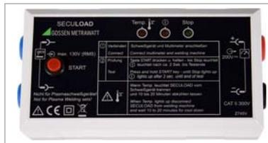
In combination with the test instrument, the test adapter is used for testing welding units in accordance with the IEC/EN 60974-4 standard. This standard stipulates that peak values for open-circuit voltage may not exceed the limit values, regardless of the utilized settings.
