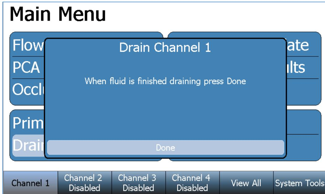
Press the **Done** key when no fluid remains in the drain line tubing.
