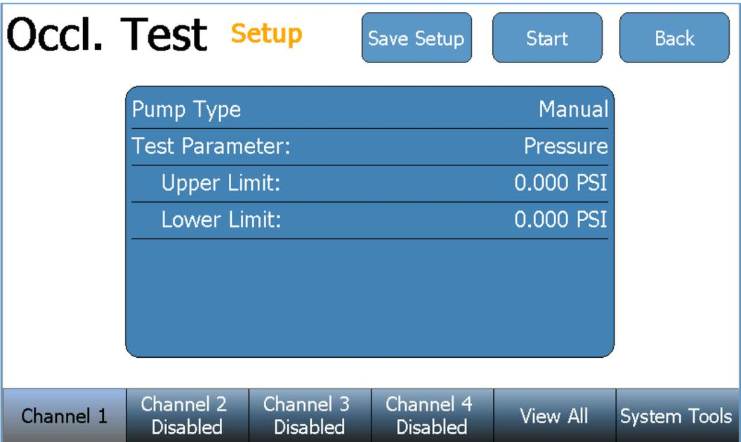
The Occlusion Test setup screen includes the occlusion test setup and control parameters. To change a setting, simply press the parameter to display the available options, select an option, or enter the desired value. Use the **Save Setup** key to save to save the current selections for use with another Channel or another SECULIFE IFPRO. See the “Loading a Test Template” section of this manual for details.
