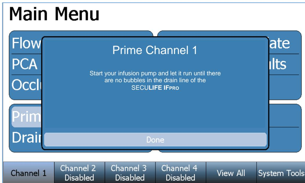
Press the **Done** key when no visible bubbles remain in the drain line tubing.
