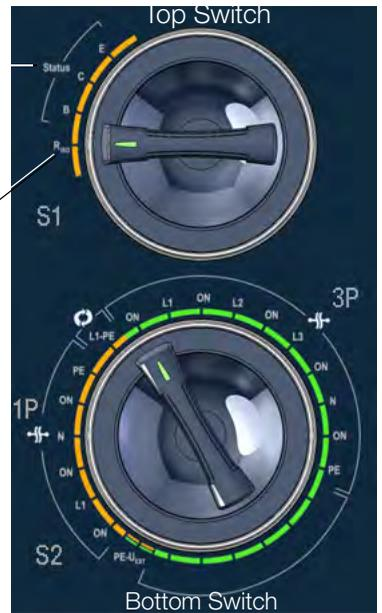
Orange switch positions: testing at single-phase, mode 2/3 cables
