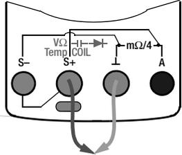
Short circuit measuring cable ends
