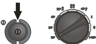
Switch the measuring instrument on. Set the function selector switch to the **2p** position.
