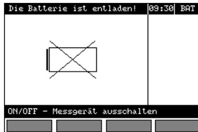
Batteries are extremely depleted – measurement is disabled.
