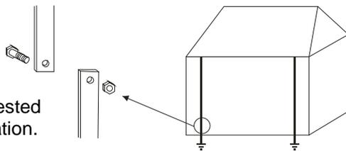
Disconnect the earthing to be tested from the installation.
