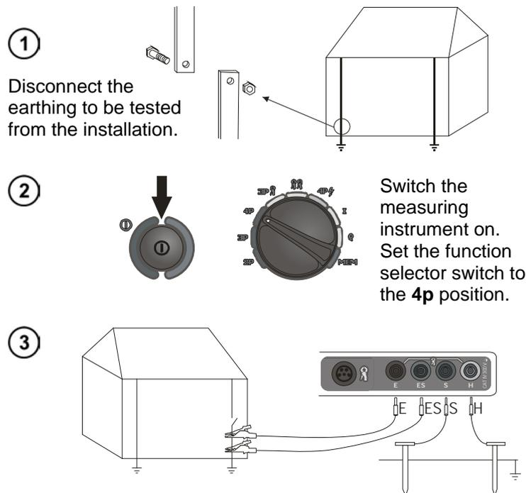
The current conducting electrode – driven into the ground – must be connected to the **H** socket at the measuring instrument. The voltage conducting electrode – driven into the ground – must be connected to the **S** socket at the measuring instrument.
