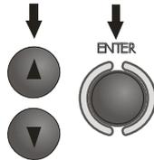
Select a frequency with the ▲ and ▼ keys. Acknowledge your selection by pressing the ENTER key.
