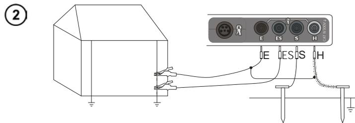
The current electrode, driven into the ground, must be connected to the **H** socket at the measuring instrument via a shielded cable.
