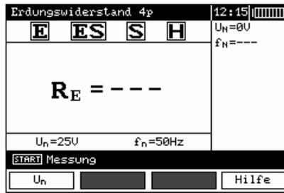
The measuring instrument is ready for measurement. Interference voltage and its frequency can be read from the auxiliary display. The line frequency selected in the menu is displayed in the settings line.
