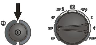
Switch the measuring instrument on. Set the function selector switch to the **3p** position.
