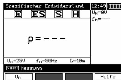
The measuring instrument is ready for measurement. Interference voltage and its frequency can be read from the auxiliary display. The following appear in the settings line: measuring voltage, line frequency selected in the **menu** and the distance between the electrodes.
