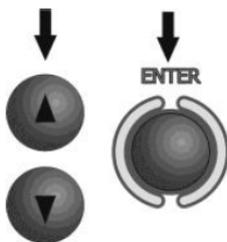
Select activation or deactivation of the GPS function with the ▲ and ▼ keys. Press the **ENTER** key to acknowledge your selection.
