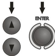
Select the desired measuring voltage with the **▲** or **▼** key and acknowledge your selection by pressing the **ENTER** key.
