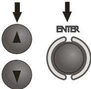
Select the desired pulse form with the **▲** and **▼** keys and acknowledge your selection by pressing the **ENTER** key.
