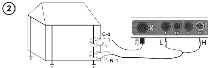
The clamps must be closed around the earthing to be tested at a distance of 30 cm from each other. The emitting clamp meter must be connected to sockets **H** and **E**, and the receiving clamp meter must be connected to the clamp meter socket.
