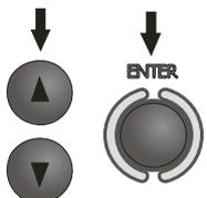
Select the desired measuring voltage with the ▲ and ▼ keys and acknowledge your selection by pressing the **ENTER** key.
