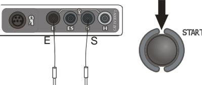
Open the measurement cables. Press the **START** key.
