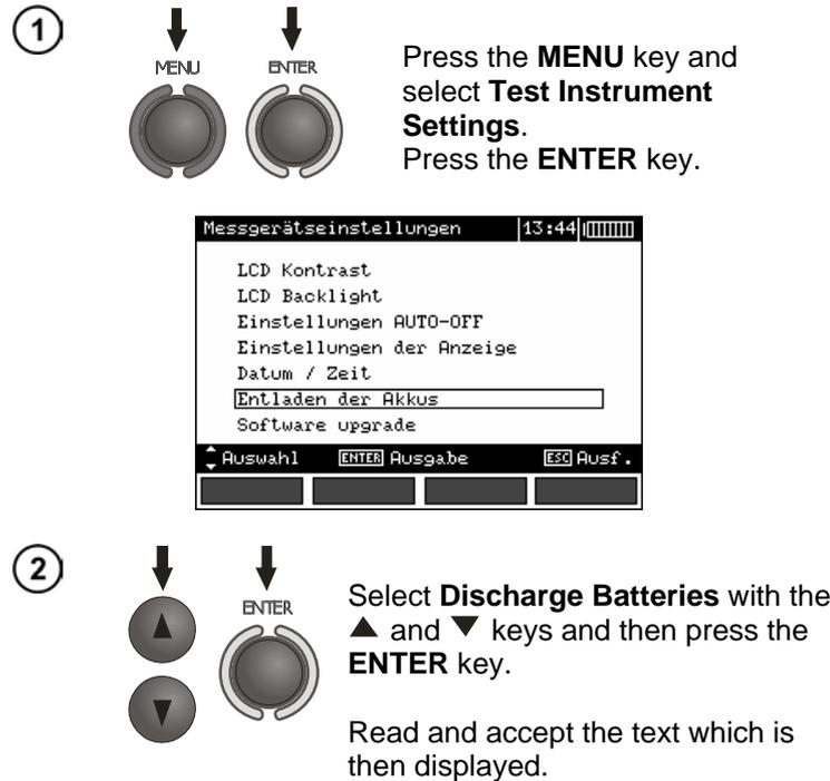
Discharging takes up to 10 hours depending on the battery pack's charge level and is indicated by the following display: **Discharging Process Status**.
