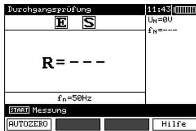
The measuring instrument is ready for measurement. Interference voltage and frequency values can be read from the auxiliary display. The line frequency selected in the menu is displayed in the settings line.
