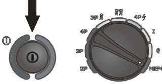
Switch the measuring instrument on. Set the function selector switch to the **MEM** position.
