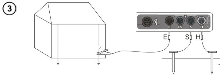
The current conducting electrode – driven into the ground – must be connected to the **H** socket at the measuring instrument. The voltage conducting electrode – driven into the ground – must be connected to the **S** socket at the measuring instrument.
