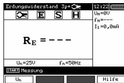
The measuring instrument is ready for measurement. Interference voltage and its frequency, as well as the RMS value of current flowing through the clamp meter, can be read from the auxiliary display. The line frequency selected in the menu is displayed in the settings line.
