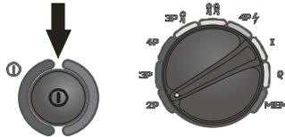
Switch the measuring instrument on. Set the function selector switch to the **2p** position.
