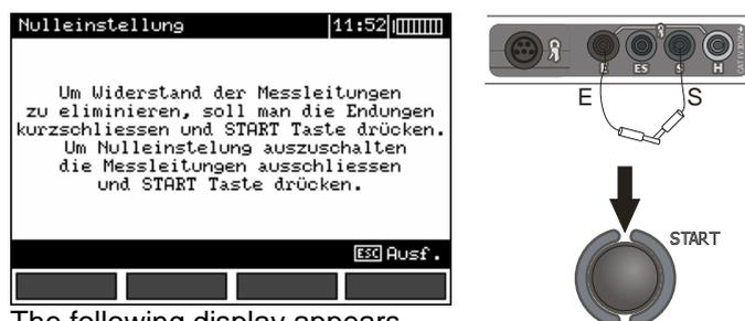
The following display appears after automatic zeroing has been completed:
