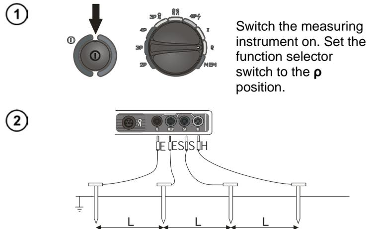
The four probes which have been driven into the ground at equal distances from each other must be connected to the measuring instrument in accordance with the illustration shown above.
