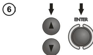
Select the desired measuring voltage with the **▲** or **▼** key and acknowledge your selection by pressing the **ENTER** key.
