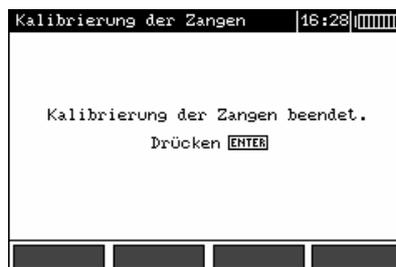
The measuring instrument determines the correction factor for the connected clamp meters. This factor remains in memory even after the measuring instrument has been disconnected from supply power, until the next time the clamp meters have been successfully calibrated.
