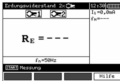
The measuring instrument is ready for measurement. Amperage of the current flowing through the clamp meters, as well as its frequency, can be read from the auxiliary display.
