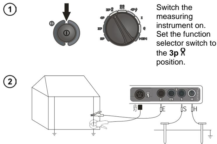
The current conducting electrode – driven into the ground – must be connected to the **H** socket at the measuring instrument. The voltage conducting electrode – driven into the ground – must be connected to the **S** socket at the measuring instrument.
