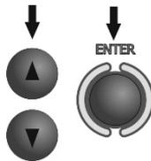
Set illumination time with the ▲ and ▼ keys and acknowledge by pressing the ENTER key.
