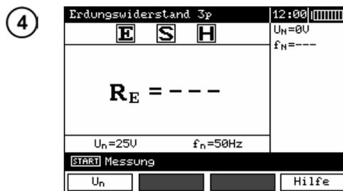
The measuring instrument is ready for measurement. Interference voltage and its frequency can be read from the auxiliary display. The line frequency selected in the menu is displayed in the settings line.
