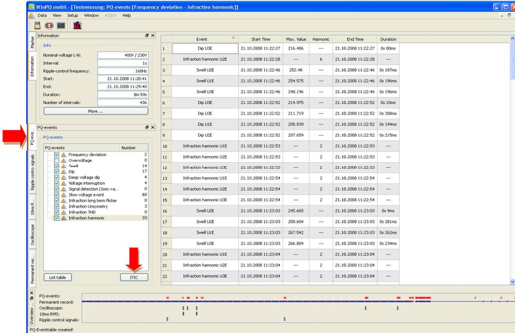
With the **ITIC** button it is possible to display all the voltage events as an ITIC representation. All deviations from the nominal voltage in duration and amplitude are displayed graphically.
