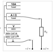
(without transient resistor!) in series with the power consumer  $\rm R_{\rm V}$  . With DC current note the polarity!
