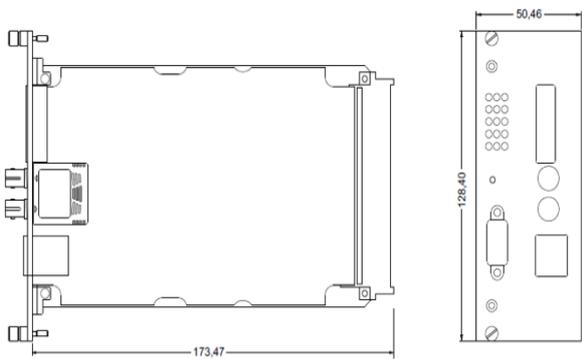
Picture 2: Dimensions plug-in module at B2 release
