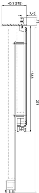
Picture 3: Dimensions plug-in module at B1 release
