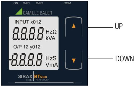
SIRAX BT5300 can be configured and programmed at site for the following: Input parameters (i.e start, end and elbow value of Input) and Output parameters (i.e as Voltage or as Current and start, end and elbow value of outputs). The front panel has two push buttons through which the user may scroll through the output screens and configure the product.
