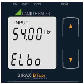
Pressing the “**Down**” key will enter the “New/Change Elbow value of the Input edit” mode.
