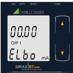
Pressing the “**Down**” key will enter the “New/Change Elbow value of the Output 1 edit” mode.
