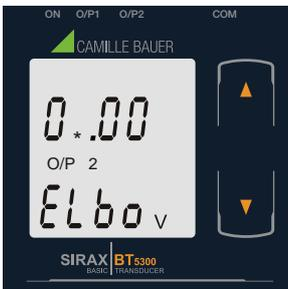
Enter New / Change Elbow value of the Output 2, first digit entered, prompting for second digit. (\*Denotes that digit will be flashing).
