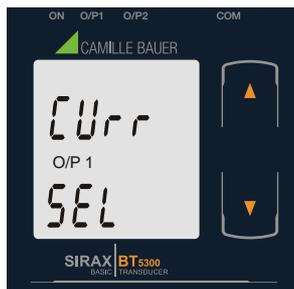
Pressing the “
