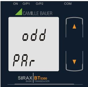
Pressing the “**Down**” key will enter the “Parity & stop bit edit” mode and scroll the value through odd: odd parity with one stop bit
