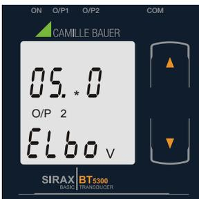
Enter New / Change Elbow value of the Output 2, second digit entered, prompting for third digit. (\*Denotes that digit will be flashing).
