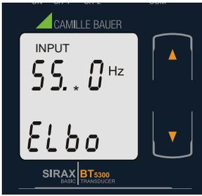
Enter New / Change Elbow value of the Input, second digit entered, prompting for third digit. (\*Denotes that digit will be flashing).
