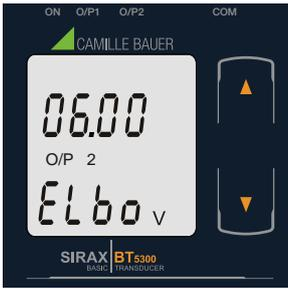
Pressing the “
