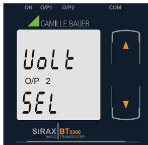
Pressing the “
