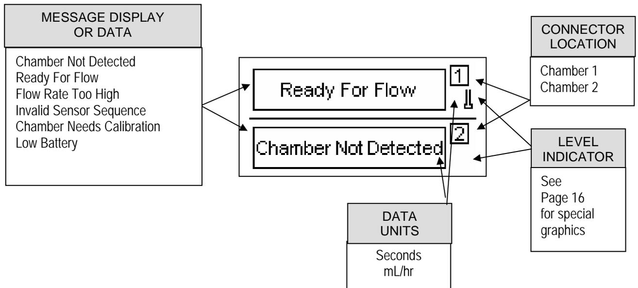
**CONNECTOR SCREEN** – The connector screen indicates the layout of the connectors at the top of the SECULIFE IF+. Also shown is the volume capacity of any connected Chambers.
