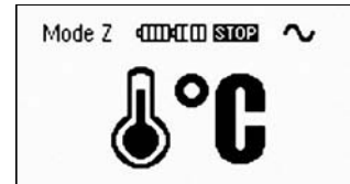
Figure 3.11: Overheating Display After Pressing the Start Key
