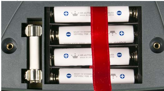
Figure 6.1: Correct Battery Polarity
