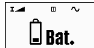
Figure 3.9: Battery Status After Pressing the START Key
