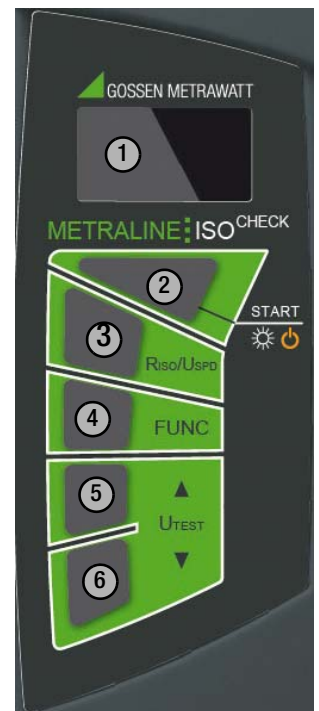
Figure 2.3: Control Panel and OLED Display
