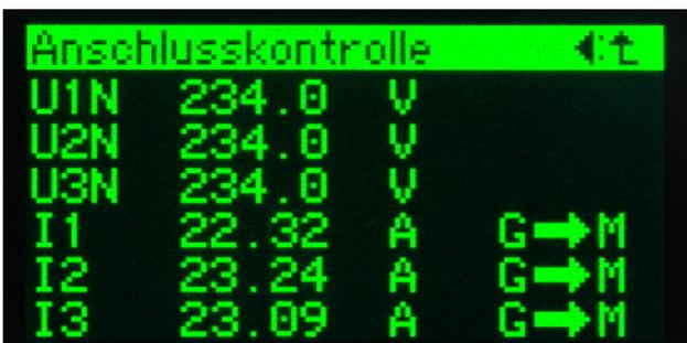
appropriate measurement displays are variable. Up to 12 different pages may be displayed. The selection is performed using the keys ▲ and ▼.
