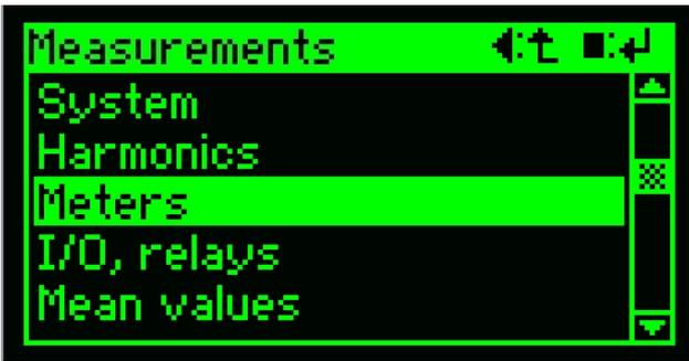
Meter contents are acquired for both the measured system as well as for analog inputs. For digital inputs it takes place only if the inputs are configured as meter inputs.
