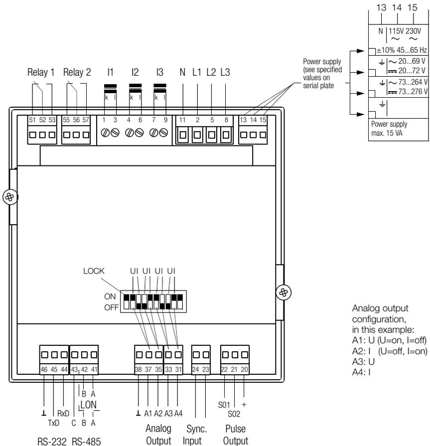
Analog output configuration, in this example:
