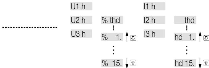
When displaying the maximum values of the harmonic, press key **P** to indicate the time and date when the respective maximum value occurred.
