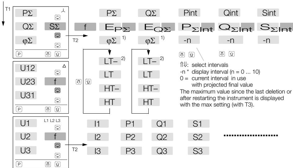
If a rotating field is established at the U or I inputs of the A2000, the neutral conductor current is displayed instead of the frequency.
