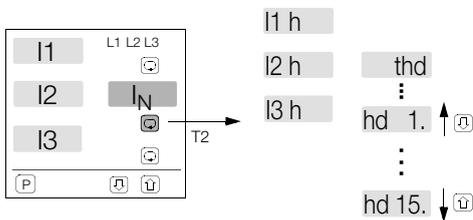
When displaying the maximum values of the harmonic, press key [P] to indicate the time and date when the respective maximum value occurred. (Function only available for version with data logger)
