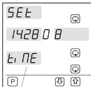
Selection and storage of hours and minutes (corresponding display blinks)
