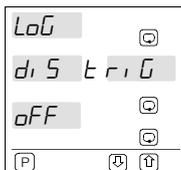
External trigger disabling when trigger source ≠ OFF
