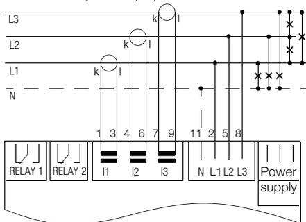
Connection with 2 current transformers in 3-wire systems (3L)
