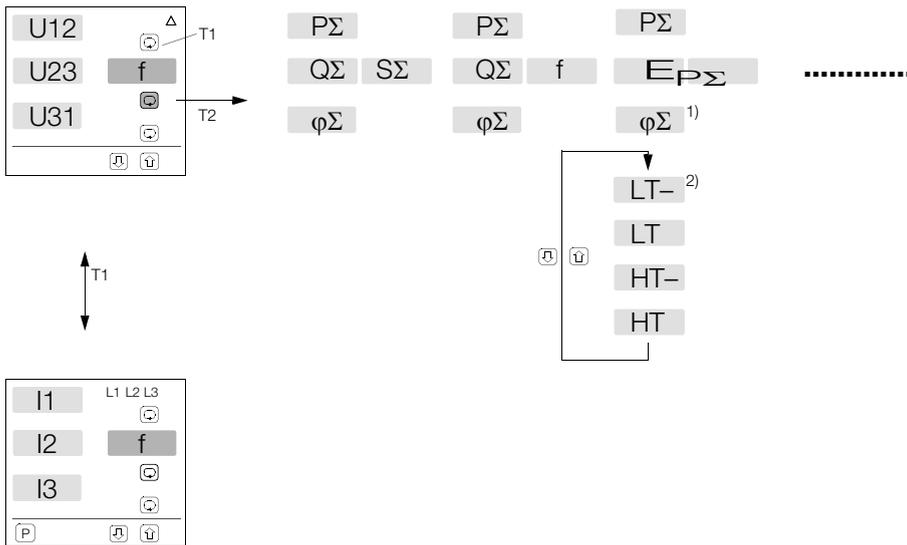
If a rotating field is established at the U or I inputs of the A2000, the neutral conductor current is displayed instead of the frequency.
