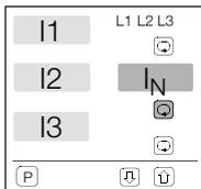
L1, L2, L3,  $\Delta$ ,  $\Delta$  and L123 comprise 6 display groups. If a given group is exited, the current display mode is stored to memory and is re-initialized when the group is queried again.
