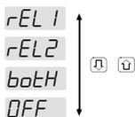
If the trigger source is set to OFF, data is recorded continuously to memory. For data logger an alarm memory is not relevant.
