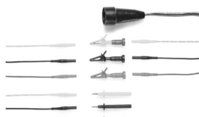
The KS 13 cable set consists of an adapter socket with 3 permanently connected cables, 3 measurement cables, 3 plug-on pick-off clips and 2 plug-on test probes. With the KS 13, the test instrument and the device under test can be
