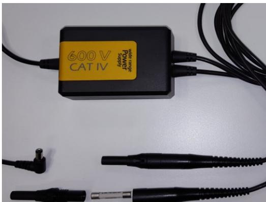
In fuse carrier only 6.3mm x 32mm, 3 A, F, fuses are allowed, with a shut-off value of 50kA. Only fuses with the identical data must be used.
