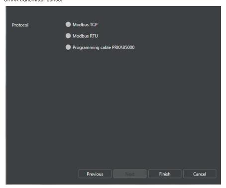
After selecting the protocol you can click finish and the new configuration is created and the configuration screen is shown.
