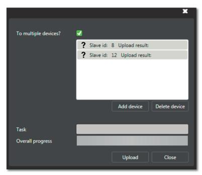
In the screenshot above 2 additional are added, slave 8 and 12. When you click the upload button now CB-Configurator will first send the changed settings to the main device and then it will start the upload for the 2 additional devices. Because CB-Configurator does not know which settings are changed for the additional devices, it will upload all settings except for the slave id and the ip-address settings.
