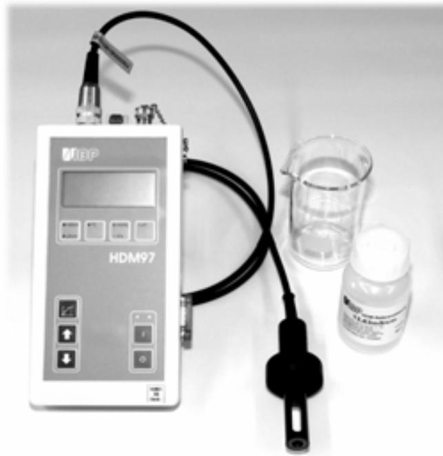
1. Press and release the **Conductivity key** to select the Conductivity channel, then press and hold the **Cal key**. The display counts down from 5 to 0. Keep the **Cal key** pressed until the instrument beeps and zero appears in the display. *If the Cal key is kept pressed for longer, it is possible to recall the standard adjustment value. Refer to the Standard Values section for more details. If the Cal key is*
