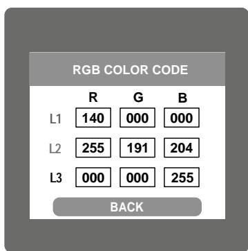
This screen allows user to set the values of Red, Green and Blue components of colors used to display the parameters of all three phases. Different colors can be assigned to each phase using combination of Red, Green and Blue component values. L1, L2 ,L3 will be set to the assigned color.
