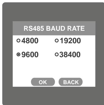
This screen allows the user to set Baud Rate of RS 485 port.
