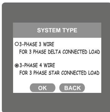
This screen is used to set the system type.
