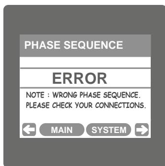
Meter shows phase rotation error if the phase sequence R-Y-B (L1-L2-L3) is not maintained. This screen indicates that Phase sequence is incorrect. User must check this screen in order to get correct readings When meter is connected.
