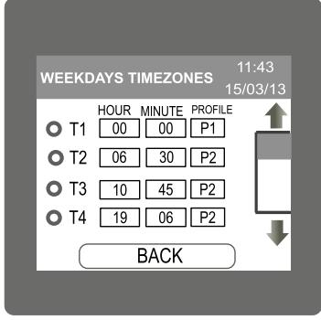
User should ensure that time zones and profile rate are assigned to all selected seasons and day types. The timezones for the day must be in sequential order and must not overlap. Minimum 1 and maximum 6 time zones can be configured. For timezone1 the default time is assigned as 00:00. User has to select a profile rate for it.
