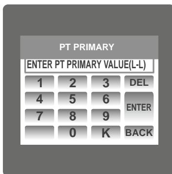
This screen can be accessed only from system parameters list menu. Here again 0 to 9 digit input keypad is provided to set value of PT Primary, & user can confirm this value with a simple touch “**ENTER**” key. “**K**” key is used to multiply value by 1000.
