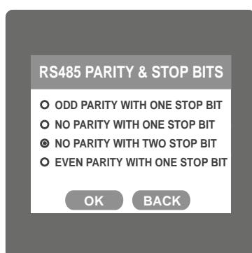
This screen allows the user to set Parity & number of stop bits. Four options: ODD PARITY WITH ONE STOP BIT, NO PARITY WITH ONE STOP BIT, NO PARITY WITH TWO STOP BITS, EVEN PARITY WITH ONE STOP BIT are displayed on screen. Touching radio button in front of particular option will select that option.
