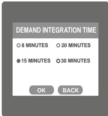
This screen is used to set the period over which current and power readings are to be integrated.
