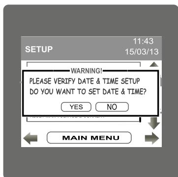
Time Of Day Setup options allows easy configuration of TOD module Every time when this option is selected it will pop up a message to ask user to verify date & time. It will ask user if he wants to set date & time. When pressed yes user will be directed to clock setup. Pressing no will continue to Time Of Day setup.
