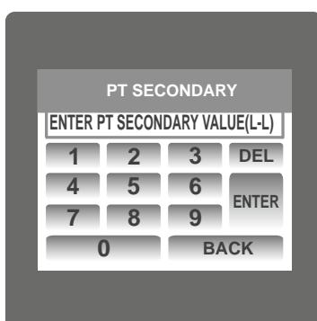
The value must be set to the nominal full scale secondary voltage which will be obtained from the the Transformer when the potential transformer(PT)primary is supplied with the voltage defined in 3.2.1.2 potential transformer primary voltage. The ratio of full scale primary to full scale secondary is defined as the transformer ratio.
