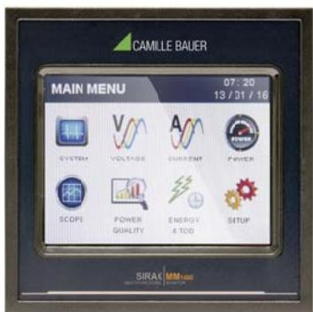
In normal operation the user is presented with one of the measurement reading screens out of several screens. These screens from particular submenu may be scrolled through one at a time in incremental order by touching the “” key and in decremental order by touching “” key on that screen. Viewing of any individual parameter with large reading (eg. shown of Line to neutral Voltage L2 in sub menu 2 screen 13) is also possible by touching that particular parameter.
