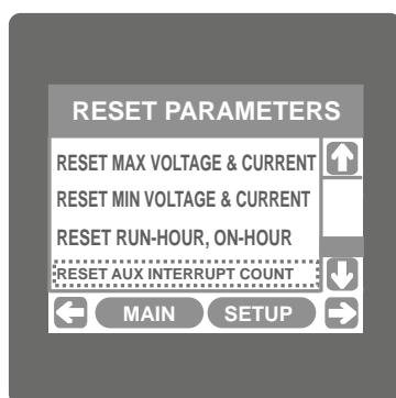
This screen is displayed after repeatedly touching “ down” key. Touching “ Up” key scrolls list in downward direction.
