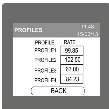
Profile contain a tariff rate that can be assign to particular timezone. Max 4 profile rate can be assign. User can assign profile rate for P1, P2, P3 & P4 between 0.001 to 299.0.
