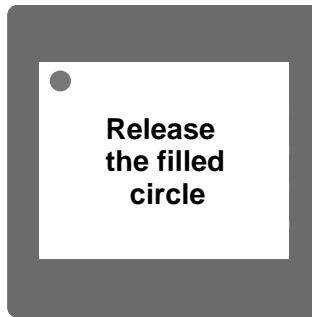
Follow the instructions displayed. Press & hold the center of the filled red circle for at least 2 seconds. Release when message for release is being displayed. For accurate results try to touch the center of the filled circle.
