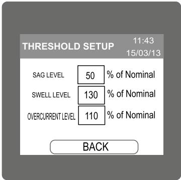
For threshold setup click on threshold setup menu. For sag level, touch the sag level menu and enter the value. The valid threshold level for sag is from 10 % to 90 % of nominal. If user enters wrong value then it will display "INVALID VALUE" and will display the valid range. Similarly threshold value for swell and overcurrent can be configured. The valid range for swell and overcurrent is 110 % to 150 % of nominal value. PT Secondary is considered as nominal value.
