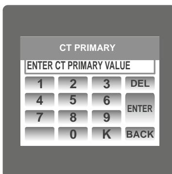
In case presently displayed Current Transformer Primary Value together with the Potential Transformer Primary Value results in a maximum power of greater than 666.6 MVA, "invalid value" will be displayed. Example: If primary value of PT is set as 692.8kV L-L (max value) then primary value of Current is restricted to 1157A.
