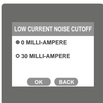
Two options, 0 MILLI-AMPERE & 30 MILLI-AMPERE are displayed on screen. Touching radio button in front of particular option will select that option.
