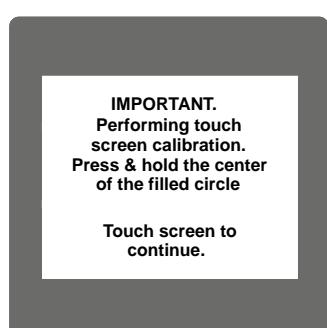
For starting touch screen calibration, touch the screen any where before power up and hold for 1 sec during starting. After that touch screen calibration will start & the message shown besides will be displayed. Touch the screen to continue.
