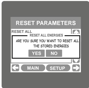
Touching on any parameter will display the confirmation dialog, now a touch on " **YES** key' will confirm the resetting of that particular Parameter.
