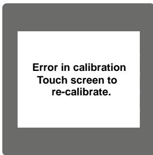
If the touch screen was not calibrated properly, "Error in calibration" message would be shown & the user will be asked to recalibrate the touch screen. In such case the meter will retain the previously stored touch - screen calibration values unless a successful calibration is being performed.
