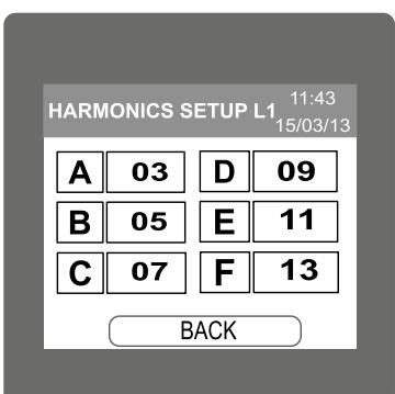
In harmonic setup, user can define the order of harmonics that user want to observe for each phase. Maximum 6 different harmonics number can be configugred at a time. For setting of harmonic, touch on the rectangle and enter the number. Valid range for harmonic no is from 2 to 56. Entering wrong value will display "INVALID VALUE" and will show the valid range.
