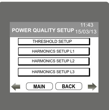
In power quality setup, user can set threshold levels for sag, swell and overcurrent detection. Also user can enter the harmonic no which user want to observe.
