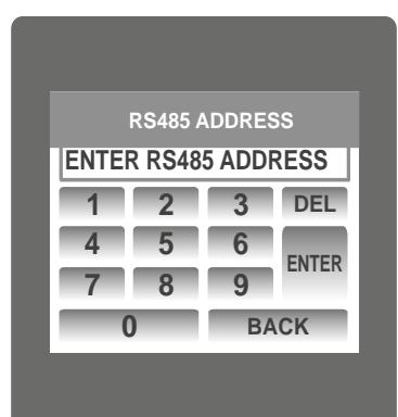
This screen applies to the RS 485 output only. This screen allows the user to set RS485 address parameter for the instrument.
