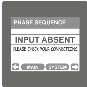
This Screen indicates that either of the phases or all three phases (Voltages) are absent.
