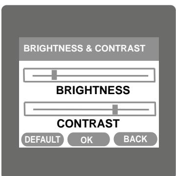
The brightness & contrast of the TFT LCD screen can be varied by the user by sliding the sliders. Touching the "OK" key will confirm the current brightness contrast setting.
