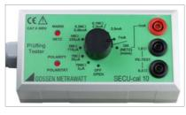
The calibration adapter is used for testing the measuring safety of test and measuring instruments by measuring protective conductor resistance, insulation resistance and leakage current.
