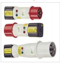
A3-16, A3-32 and A3-63 three-phase current adapters allow for trouble-free connection of testers to 5-pole CEE sockets. The three models have different sized plugs which correspond to 5-pole CEE sockets with 16 A, 32 A and 63 A nominal current. Phase sequence is indicated with signal lamps. Testing for the effectiveness of protective measures is con-
