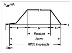
The test instrument generates a DC residual current which saturates the magnetic circuit of the RCCB.
